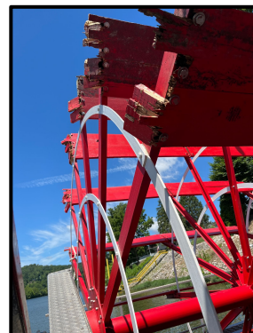
Photos Left to Right: The JENNY B, between the HOBBY III and MISS STERLING, gets towed to the Eads landing for repairs. A look at broken bucket plates that need repaired along the wheel. Capt. Kris Eads and Capt. Rick Burden at work putting on the new wheel shaft.
