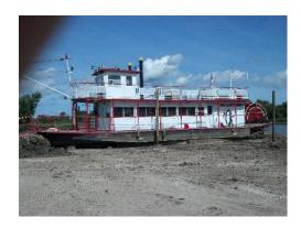
To get it there we built a levee around the boat and pumped water into the pond and floated it over onto the blocks. Then broke the levee letting the water go out. Total cost \$100 bucks for fuel. I own the dozer, excavator, and water pump only took 3 hours.
